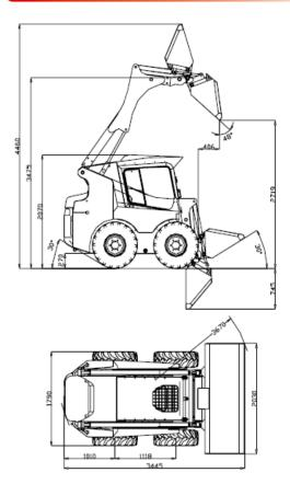
Loaders have hydrostatic transmission and a quality hydraulic system from REXROTH and can operate even in the hardest working conditions. Double filtration of hydraulic oil with constant electronic control of the cleanliness of the hydraulic filter ensures trouble-free operation and extend the life of the loader. Machine operation is done via joystick.
