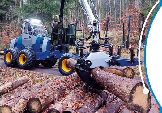
✓ High pulling force of 120 kN✓ Cranab hydraulic crane
